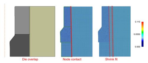
Shrink fit enhancements were introduced to the die stress analysis workflow. A new definition option automatically selects nodes based on contact at the shrink fit interface. The system also allows the shrink fit magnitude to be set to the detected interference between the contacting geometries. These automations (above) will simplify setup procedures for those modeling large assemblies.
