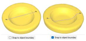
An updated state variable between two points tool (left) allows tracked points to fit to a surface and follow material flow. Options were added to snap points to an object boundary, specify multiple point groups and define patterns of points.
