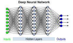
For example, a DNN model was trained on the steel flow stress definitions in the DEFORM material library. A beta version of this trained model is now accessible, within the material library, for predicting flow stress based on steel chemistry.
