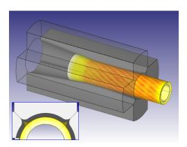
Notable changes were made to the Cogging template. The pass table now supports Boolean cropping of brick meshes between passes. It also supports scheduling of reheats between passes. As part of this change, adaptive reheat settings were consolidated with the new pass table reheat options. Other Cogging template enhancements include support for multi-pass infeed swaging (GFM), as shown on the left.
