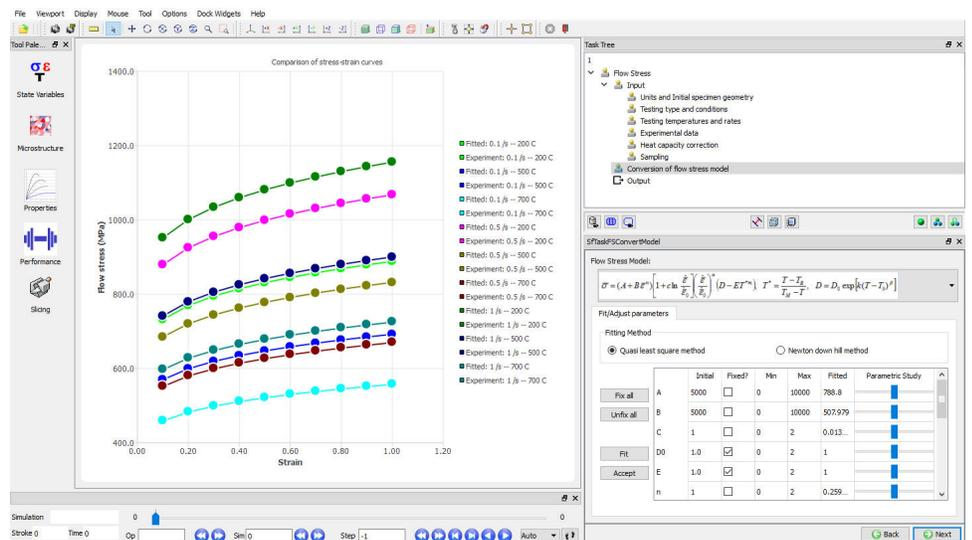
Integrated Computational Materials Engineering (ICME) is a modeling effort to relate microscale features (voids, grains, precipitates, etc.) to component-scale products and processes. The goal of ICME is to understand critical process-structure-property relationships in engineered materials. Unfortunately, simulating microscale behaviors directly within a macroscale model is, in many cases, impractical due to the time and effort that would be required.
