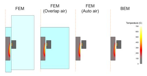
2D FEM models have a slight edge over 2D BEM models (above; right) in terms of accuracy. In the example case shown above, the best combination of accuracy and ease-of-use are provided by the overlapped and automatically-generated (hidden) air mesh FEM models. The automatically-generated air FEM model and the BEM model took the least time and effort to create.
