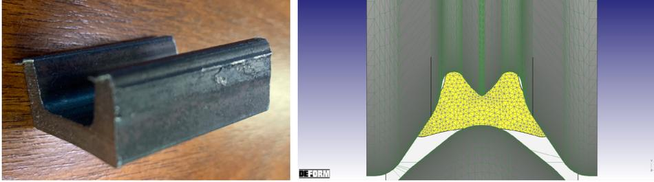
Russula used DEFORM to troubleshoot the original pass sequence and test potential redesigns. The steel producer had encountered not one but many issues while rolling the UPN 30 channel. DEFORM predicted the voids and overfill that were seen in the actual product. After this validation, subsequent designs were tested in DEFORM to ensure proper fill and eliminate defects.
