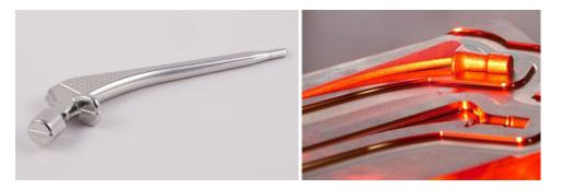
Orchid uses DEFORM-3D to couple the die designers' experience of historical forming practices with a finite-element metal flow simulation. The analysis shows if the die cavity will fill correctly and whether there is a risk of defects and nonconforming material. After the simulation runs, the die designers can adjust the die and billet geometries to improve material flow and reduce strain before the die is ever cut.
