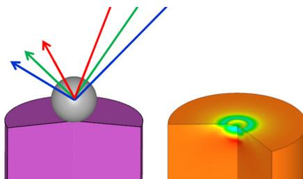
At a larger scale, process parameters such as workpiece rotation, the shot spray zone and movement are considered. All of this information is utilized to predict residual stress response and shot peening coverage at the part level.
