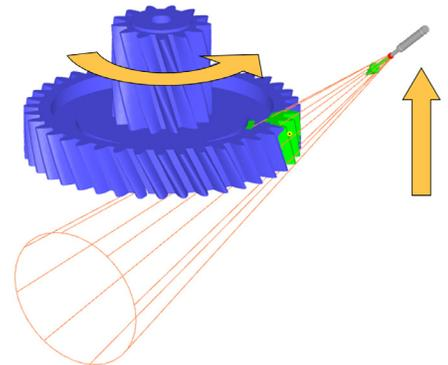
The shot peening of this gear can be modeled by following an easy-to-use, wizard-based template. The user is guided through the workflow to import CAD models and mesh the gear geometry. Objects that might impede the shot hitting the gear, providing a shadowing effect, could also be added.
