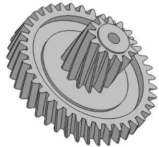
It is common for such a gear to spin during the peening process, with the spray nozzle moving up and down while firing the shot.
