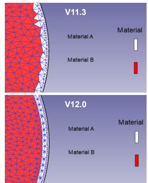
New local remeshing methods allow users to remesh a specific portion of the work-piece, rather than the entire part. State variables and geometry outside of the local zone thus remain unmodified. This benefits applications that require fine detail but involve many remeshes, such as in machining (bottom). Here, a user-defined window, which follows a cutting tool, defines the remeshing zone.
