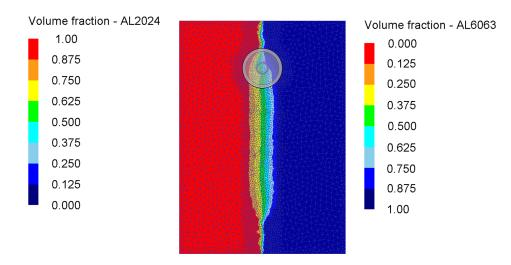
Applications of DEFORM to FSW, using the default implicit Lagrangian method, were first published as early as 2001 (2D) and 2006 (3D). An Arbitrary Lagrangian-Eularian (ALE) based method for solving FSW models was recently introduced in V11.2. Both methods allow users to evaluate the impact of material type, plate thickness, tool design, plunge depth, rotational speed and feed rate on the final welded joint.
