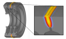
The quality of the weld joint is dictated by the applied axial pressure, initial flywheel RPM and energy, interface temperature. upset distance, flash and residual stress. DEFORM models allow users to optimize these process parameters, for a desired response, on the computer. New shapes, sizes and materials can thus be evaluated with less trial and error.
