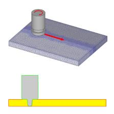
Understanding the thermomechanical behavior of this process is critical. DEFORM models have been used to predict metal flow, accumulated strain, temperature, defects and loads in the process. Advanced analyses have revealed material mixing behavior (below) and resulting microstructure.
