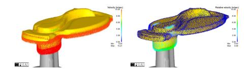
The plot show above, at right, illustrates the new "Relative Velocity" state variable. To use this state variable, a reference object must first be defined. The velocity of this reference object is subtracted from the absolute velocity field of the workpiece. The difference represents the relative velocity due to material deformation.
