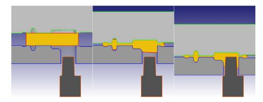
Such rigid body motion has typically made analysis of the velocity distribution difficult. Prior versions of DEFORM have only included the (absolute) "Velocity" state variable. The plot shown below, at left, demonstrates what absolute velocity looks like when the part undergoes significant rigid body motion. The rigid body velocity field overwhelms the more subtle local velocity contributions.
