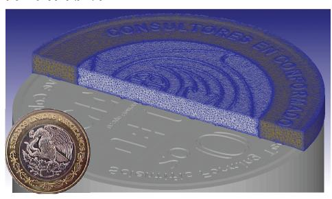
The die used in this coining process had extensive engraved text and other fine details. In order to investigate the stresses in the die, a large number of elements was required. The die was meshed using 1.9 million elements. A decoupled die stress analysis was run. The image below shows the effective stress in the die (red is higher). The close-up view shows the mesh resolution in this model. Note the resolution around the text.
