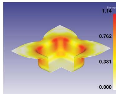
In sheet metal, the generally accepted predictor of fracture or tearing is known as a Forming Limit Diagram. A forming limit diagram plots major and minor strain directions on an X-Y graph. A curve represents the forming limit. Combinations of major and minor strain which lie above the curve represent likely tearing. Those below the curve represent a safe region.
