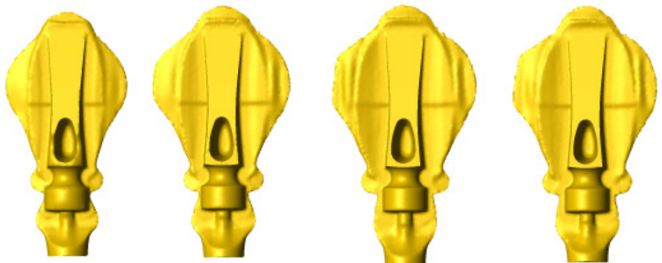
The influence of hammer stiffness is shown in the predicted finish forging results (above). Fill and flash increase as stiffness increases (from left to right). At the highest stiffness, the shape looks good but the blows are under-predicted.
