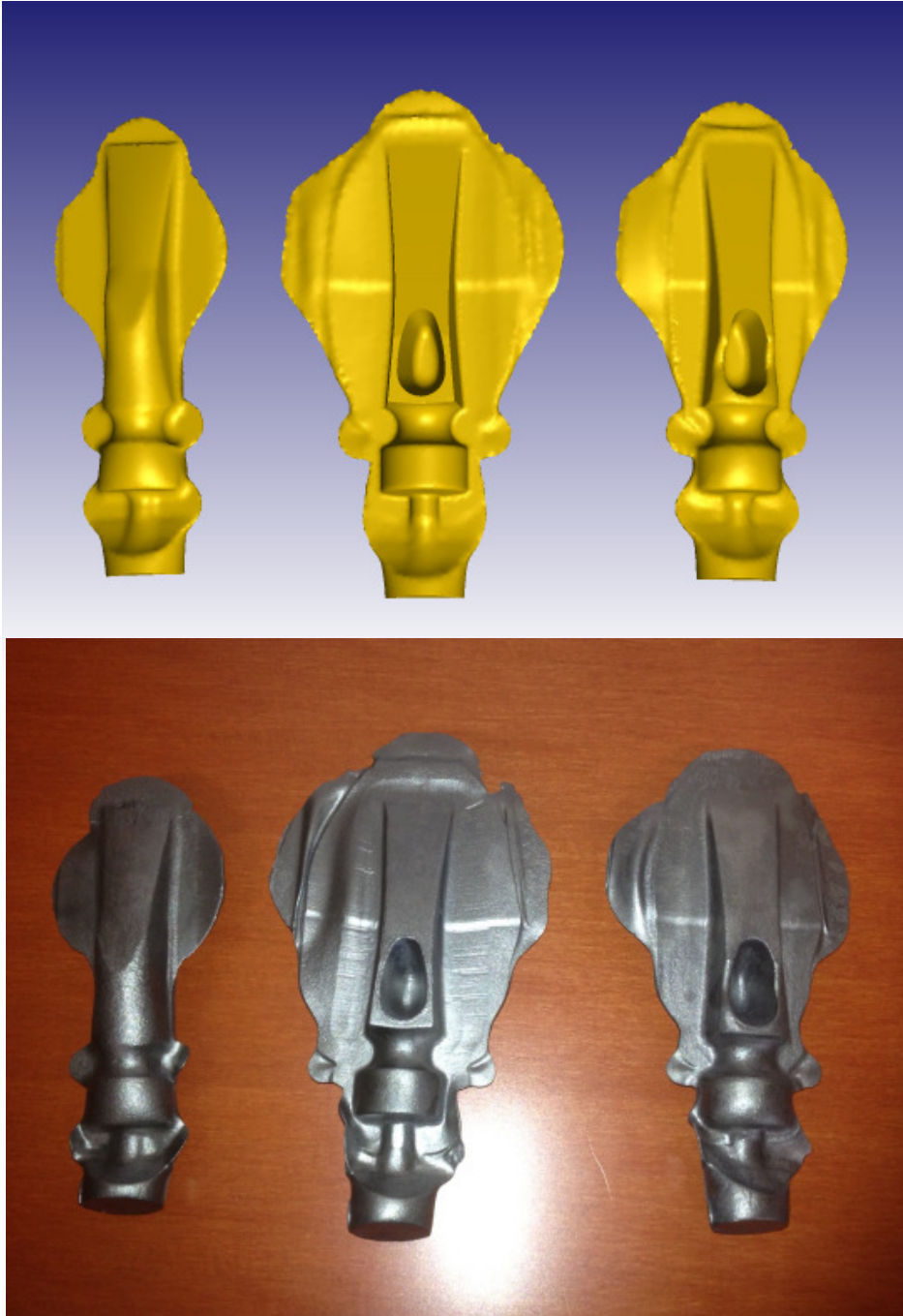
Simulation results showing the predicted bust, finish and block forgings when hammer stiffness was set to 50,000 klb-in (top). Through correlation it was determined that this stiffness provided the best match to the actual forgings (bottom).
