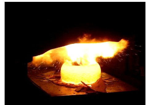
The coal dust is applied to the workpiece prior to piercing (left), resulting in a controlled explosion (right) that 'assists' with retracting the punch.
