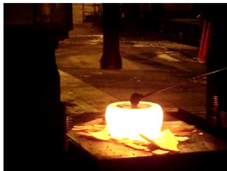
The coal dust is applied to the workpiece prior to piercing (left), resulting in a controlled explosion (right) that 'assists' with retracting the punch.
