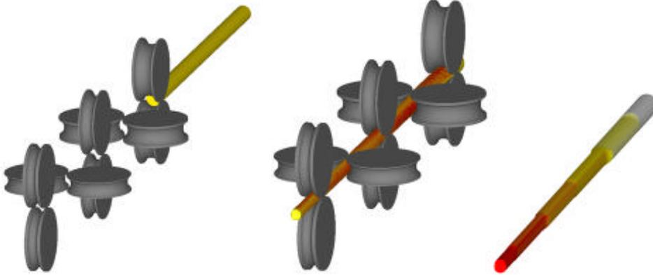
An automatic stopping criterion has been added to recognize the completion of a rolling pass. Inertia is considered so that the part will continue moving after coming out of the roll gap. In addition, table objects can now transmit frictional forces to the workpiece. This helps to drive the material into the roll gap and stabilize the solution as the workpiece exits the rolls.
