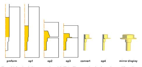
The cold forming bolt progression with 2D to 3D conversion is shown above. After three 2D forming operations the workpiece was converted to 3D (60 degree section) for the final operation. Mirroring was used to display the full hexagonal bolt.
