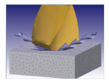
The **A**utomatic **M**esh **G**enerator produces an optimized mesh system, with local element size control based on the specific process being analyzed. This facilitates the enhanced resolution of geometric features while maintaining good control of the overall problem size and computing requirements. A user-defined local mesh definition provides advanced users with a flexible control to meet their unique requirements.
