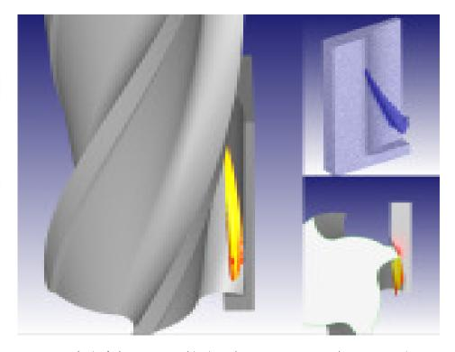
DEFORM-3D includes a very sophisticated postprocessor. Each postprocessing session is capable of displaying up to six coupled viewports. The mesh, shape, load-stroke curve, effective strain and sliced section of the workpiece are displayed in the above illustration. It is easy to compare two simulations with slightly different parameters.
