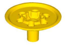
The simulation accurately predicted the wear pattern seen in production (red is higher wear - below). The wear on the protrusion would be intuitive to most experienced forging designers. On the other hand, the half-moon shaped wear is less intuitive.
