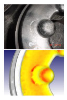
From a productivity standpoint, the production process offered room for improvement. The large deformation in the second station resulted in a high forging load. This prevented parts from being formed in stations 1 and 3 at the same time.
