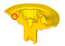
A modified "round" preform was developed to eliminate the lap. The simulation results were very promising. There were no defects, die fill was as expected and the die wear was reduced significantly.
