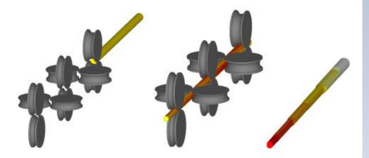
An automatic stopping criterion has been added to recognize the completion of a rolling pass. Inertia is considered so that the part will continue moving after coming out of the roll gap. In addition, table objects can now transmit frictional forces to the workpiece. This helps to drive the material into the roll gap and stabalize the solution as the workpiece exits the rolls.
