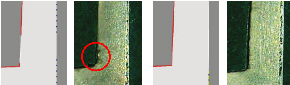
The DEFORM simulation (left) depicts underfill without venting. Die contact is shown as a red line. The underfill on the actual part is shown on the right. Note the subtle void at the corner of the punch (red circle).
