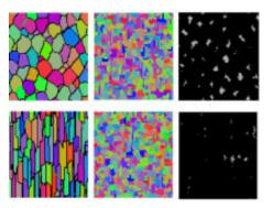
In this example, two different starting microstructures (equiaxed - top left & elongated - bottom left) are shown. The final microstructures are shown in the center. The unrecrystallized grains (gray) are shown on the right.
