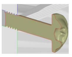
Slicing can be a useful tool when investigating thread unfill.
