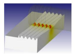
The effective stress (red is higher) is shown on this thread rolling die near the end of the forming process.
