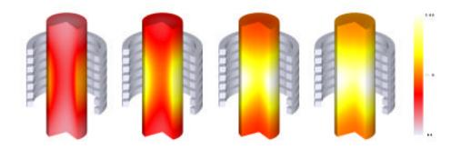
After heating, the center rod temperature was predicted as 866C (1500F).
