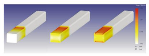
Figure 6: Contours of effective strain are shown as the roll pass progresses (from left to right). Red indicates a higher level of effective strain in this image.
