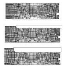
A sequence of machining operations which ensures that the final component is produced to the required tolerances was developed in a joint project by Scientific Forming Technologies Corporation, GE Aircraft Engines, Air Force Research Laboratory, and NASA. This machining sequence was created using a simulation procedure that can predict distortions created during the machining process.
